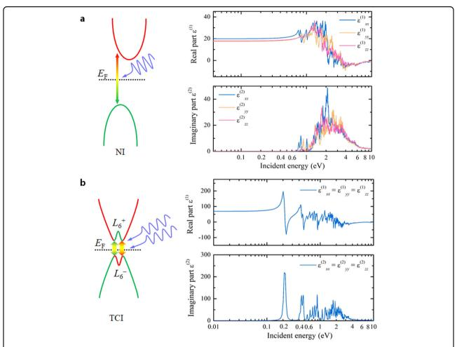
Fig. 3 Topological contrasting optical feature. Optical responses of a Pnma-SnSe and b  $Fm\overline{3}m$ -SnSe. We show the schematic optical response in the left panels. In the right panels, we show the DFT-calculated real part and imaginary part of the dielectric function along the x-, y-, and z-directions.
