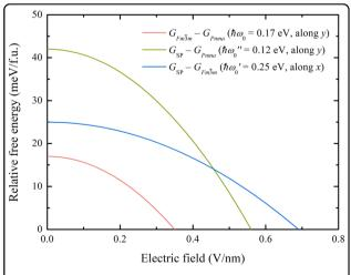
Fig. 4 Free energy difference as a function of LPL electric field magnitude. SP denotes the transition saddle point.
