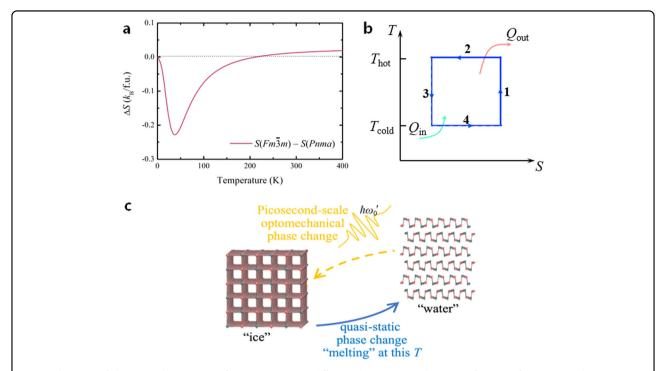
**Fig. 5 Schematic of the optocaloric process for SnSe. a** Entropy difference between two phases as a function of temperature. **b** Entropy-temperature (*S-T*) in a Carnot thermodynamic cycle. **c** Phase-change cooling cycle, that is significantly different from the Carnot cycle. Here solid lines denote quasi-static processes, whereas dashed line denotes out-of-thermal-equilibrium process.
