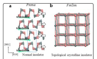
**Fig. 1 Atomically geometric phase transition of SnSe.** Geometric structures of the SnSe compound in the **a** layered *Pnma* and **b** rocksalt  $Fm\overline{3}m$  phases. In **a**, empty arrows represent the spontaneous electric polarization of each layer, and green arrows show the translation direction of each layer to form the  $Fm\overline{3}m$  phase. The blue dashed rectangle represents the simulation supercell.
